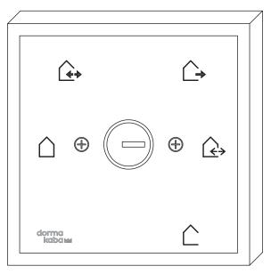
The unit is switched off. In the case of units with the optional locking mechanism, the door is electromechanically locked.
